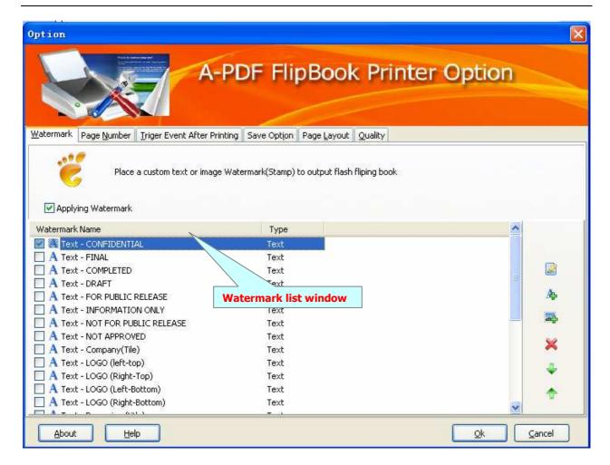
The watermarks for applying to **FlipBook document(s)** are listed in the Watermark list, where you can find text and image Watermark items list in here, you can apply watermark by marking one or multiple Watermark items checked, the watermark items which checked will to be applied to Output **FlipBook document(s)**
